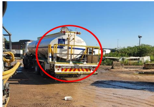
Water wastage at the Springfield filling point (water tanker drove off with its lid open)
